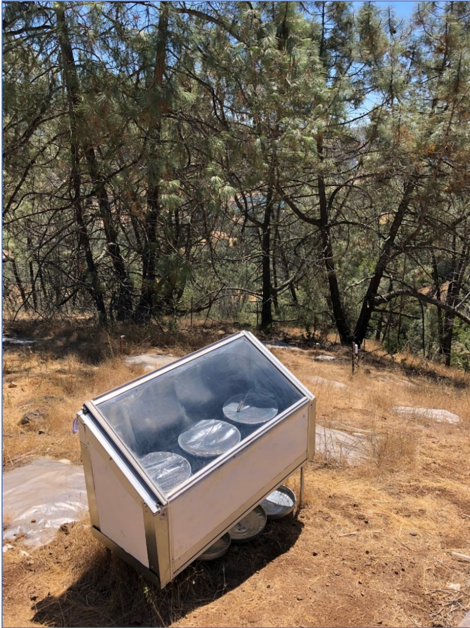
PHOTO 3. Solar oven baking contaminated soil in the Pine plot. Photo date: July 10, 2018.
