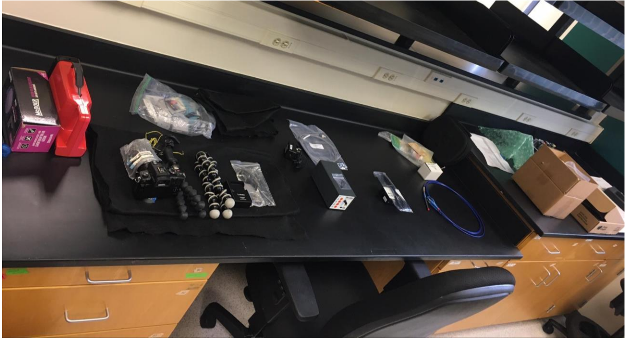
Photo 3. Flower color quantification for high throughput phenotyping. From left to right: UV light sources, UV camera and accessories (e.g., tripod), FLAME UV-Vis spectrophotometer and light source (gray box with white face) and detection probe (blue circular fiber optic cable).
