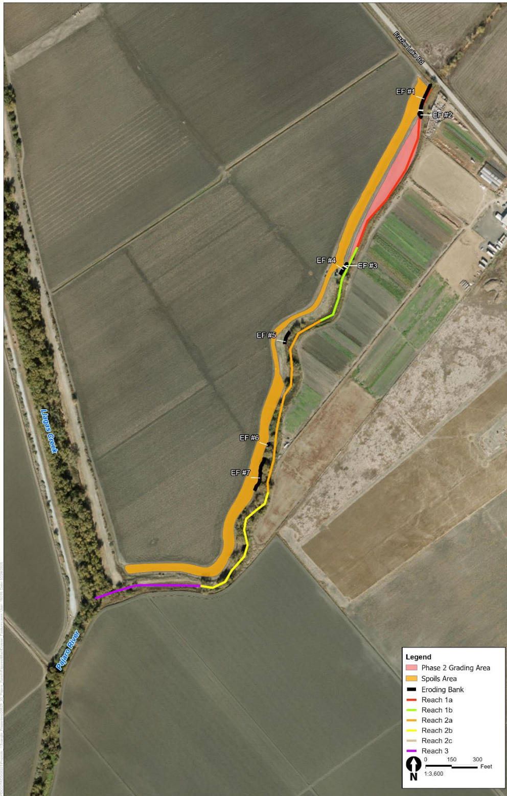
Figure 2 Pajaro River Erosion Feature Location
