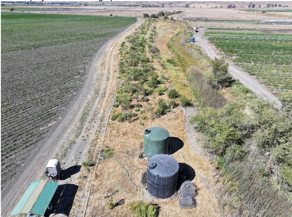
Aug. 2025: Post-grading/planting showing establishing riparian forest and developing seasonal wetland/marsh complex on right bank of the Pajaro River channel.
